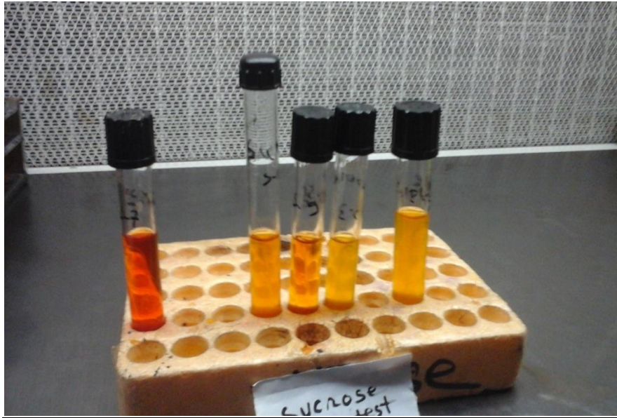
Figure 14: Sucrose test result. Left showing negative control. Right showing positive results
