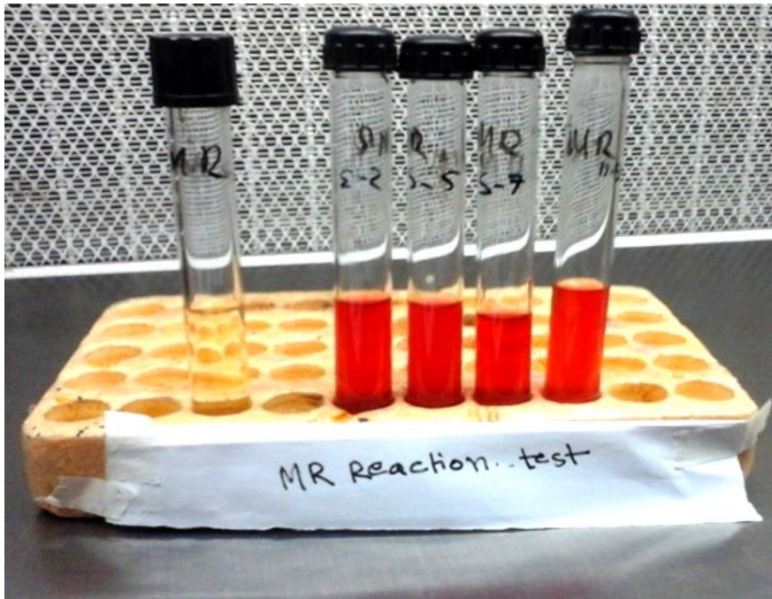
Figure 5: Methyl Red (MR) test positive result and left showing and a negative
