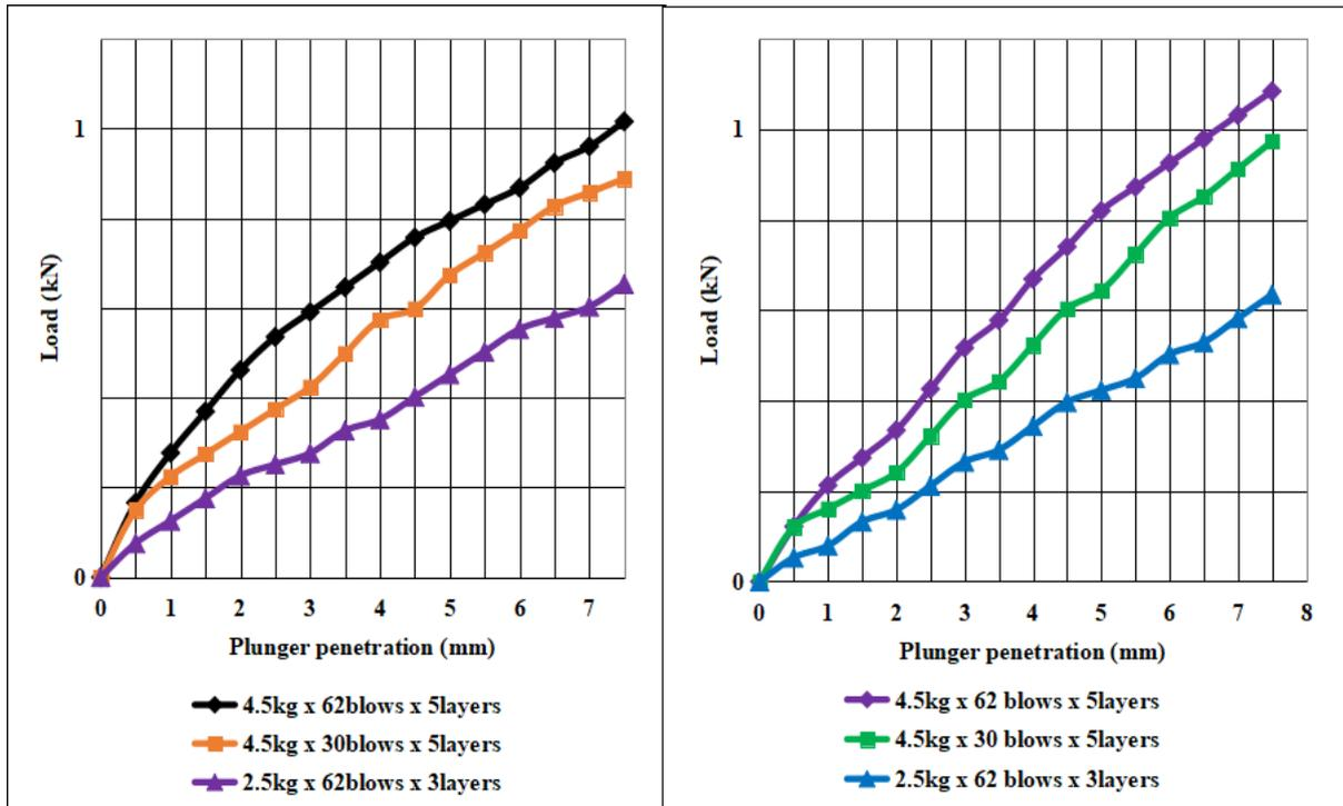
**Figure B2:** Penetration resistance of Mlimanyoka clay for 8 days soaking time (left) and 12 days soaking time (right).
