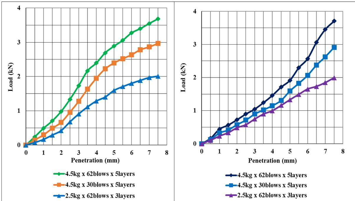
Figure B4: Penetration resistance of Ituha cinder for 8 days soaking time (left) and 12 days soaking time (right).
