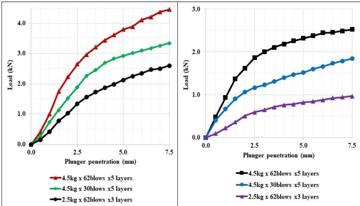
Figure B8: Penetration resistance of 64Ci27Po9Cl for 8 days soaking time (left) and 12 days soaking time (right).
