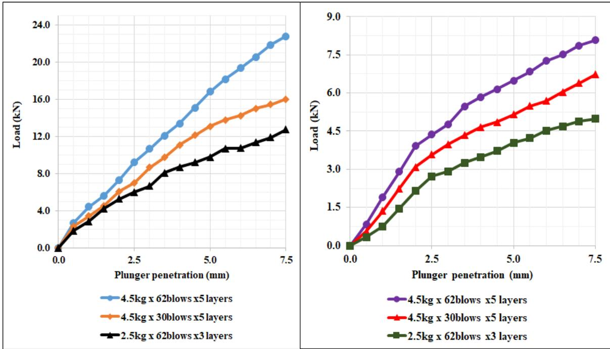
Figure B7: Penetration resistance of 64Ci27Po9Cl for 0 day soaking time (left) and 4 days soaking time (right).
