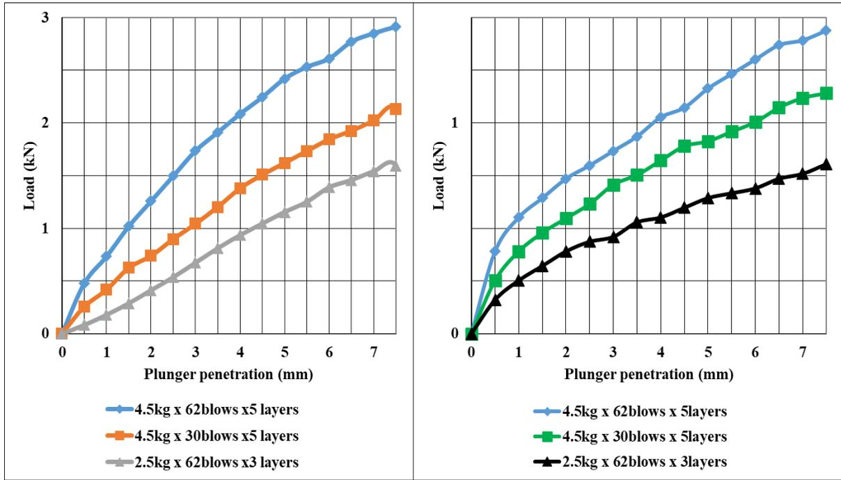
**Figure B1:** Penetration resistance of Mlimanyoka clay for 0 day soaking time (left) and 4 days soaking time (right).
