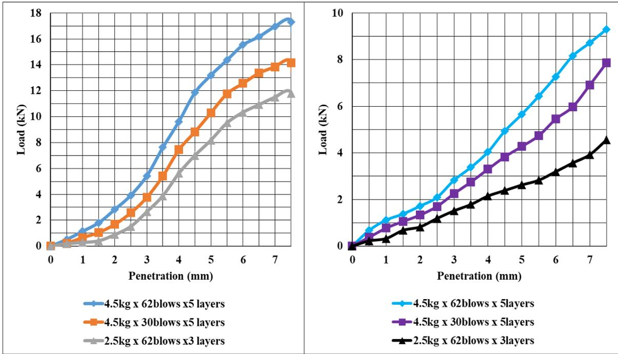
Figure B3: Penetration resistance of Ituha cinder for 0 day soaking time (left) and 4 days soaking time (right).
