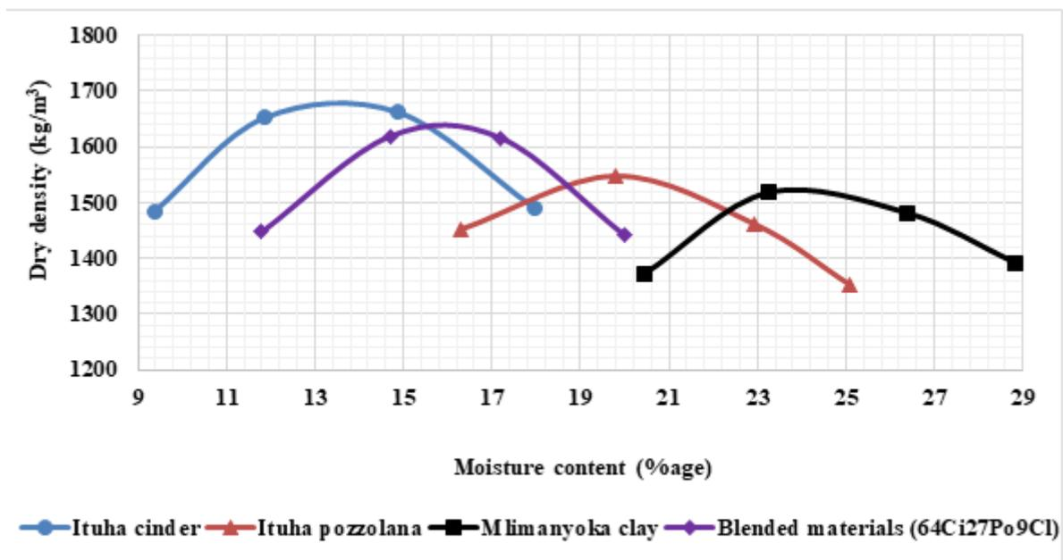
Figure 3.3: Compaction Curves of Soil Materials.
