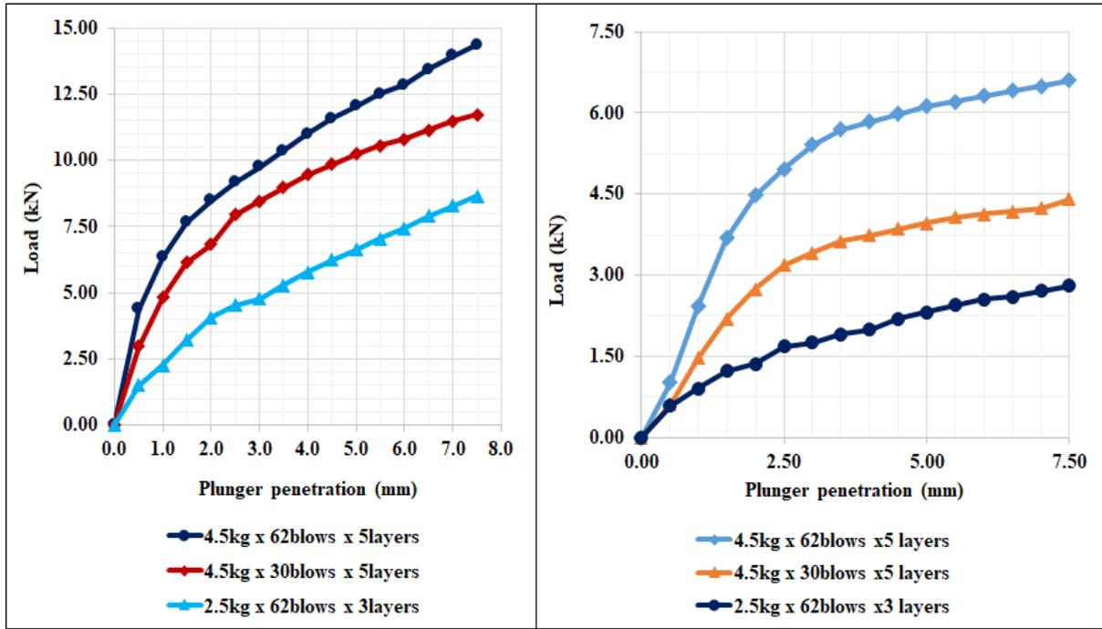
Figure B5: Penetration resistance of Ituha pozzolan for 0 day soaking time (left) and 4days soaking time (right).
