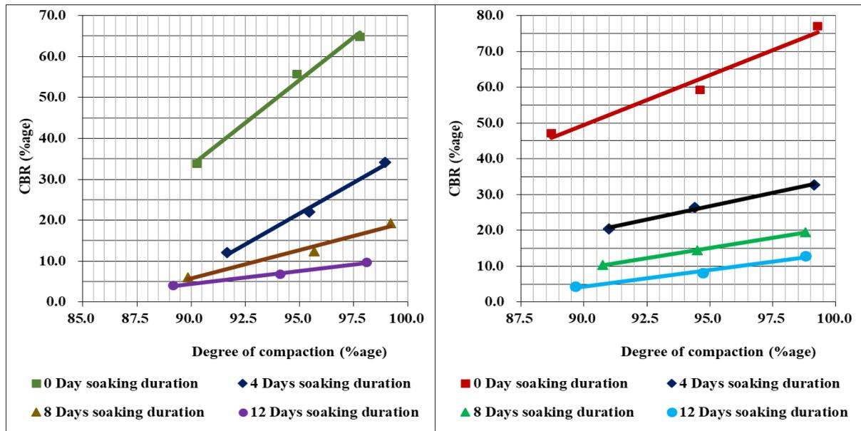
Figure A2: Three points CBR values for Ituha pozzolan (left) and Blended samples (64Ci27Po9C1) (right).
