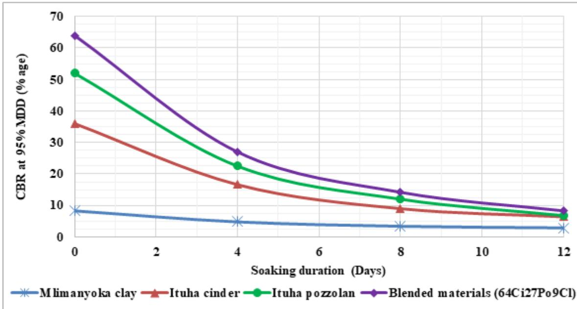
Figure 3.4: Variation of CBR of soil samples at 95%MDD with soaking days.
