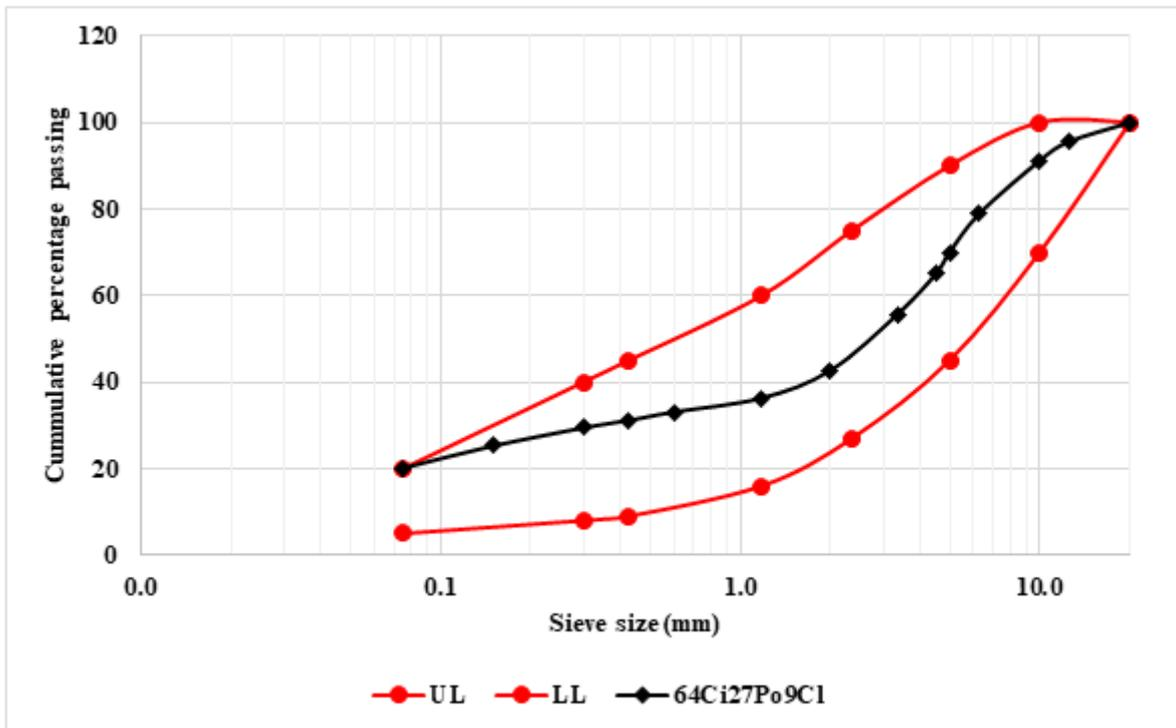
Figure 3.2: Particle Size Distribution Curves of Blended Materials.
