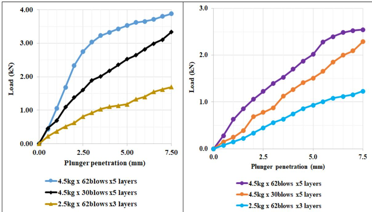
Figure B6: Penetration resistance of Ituha pozzolan for 8days soaking time (left) and 12days soaking time (right).
