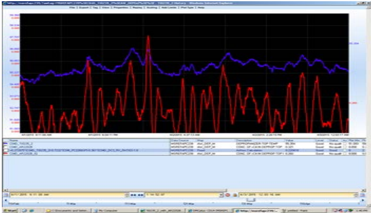
Figure 2: Existing IQ (AR2202B_IQ) vs DE-Propaniser tower top temperature (TI0235_2) changes.
