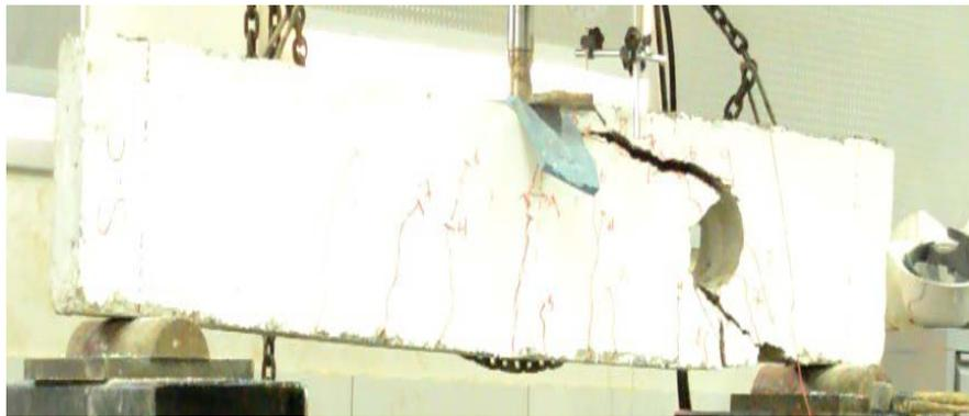
**Figure 12:** crack pattern for beam S-C
