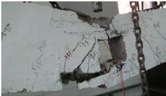
**Figure 18:** Crack pattern for beam F-R-N
