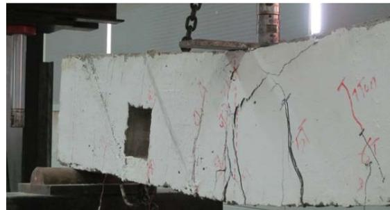
**Figure 19:** Crack pattern for beam S-R-N
