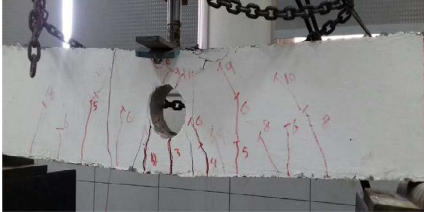
**Figure 9:** Crack pattern for beam F-C
