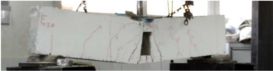
**Figure 7:** Crack pattern for beam F-R-2V
