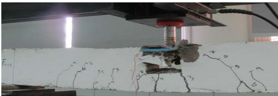
**Figure 8:** Crack pattern for beam F-R-1.5H
