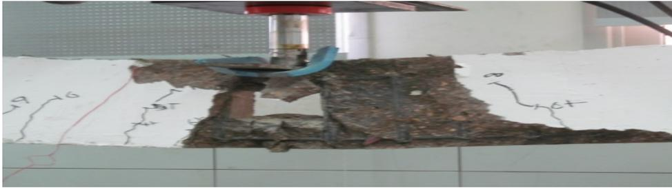
**Figure 6:** Crack pattern for beam F-S
