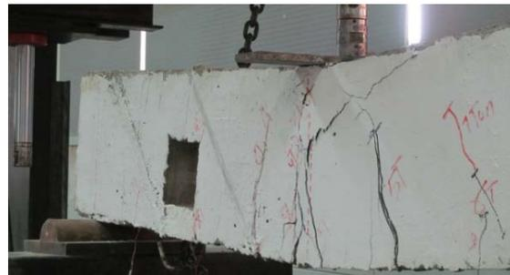
**Figure 19:** Crack pattern for beam S-R-N
