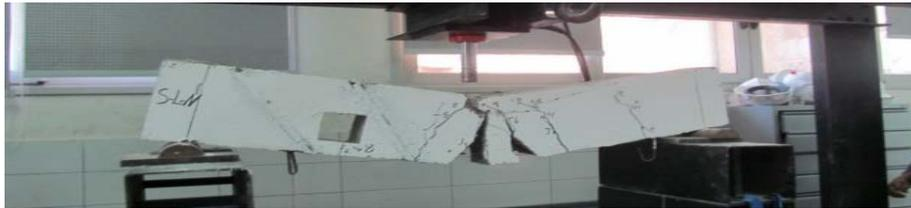
**Figure 17:** Crack pattern for beam S-L-N
