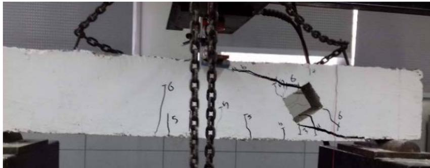
**Figure 10:** Crack pattern for beam S-S-45
