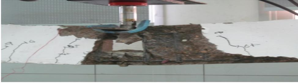
**Figure 6:** Crack pattern for beam F-S
