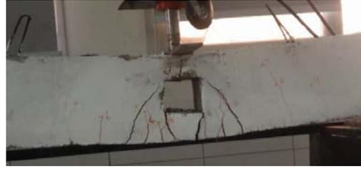
**Figure 14:** Crack pattern for beam F-R
