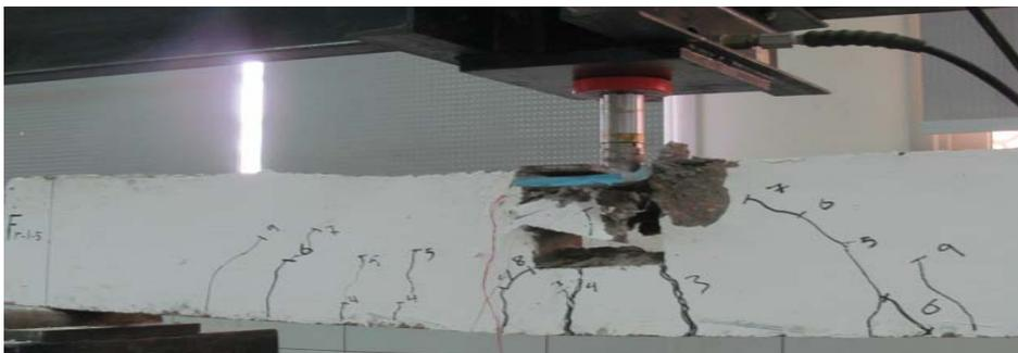
**Figure 8:** Crack pattern for beam F-R-1.5H
