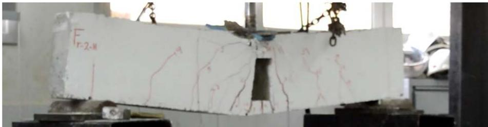
**Figure 7:** Crack pattern for beam F-R-2V
