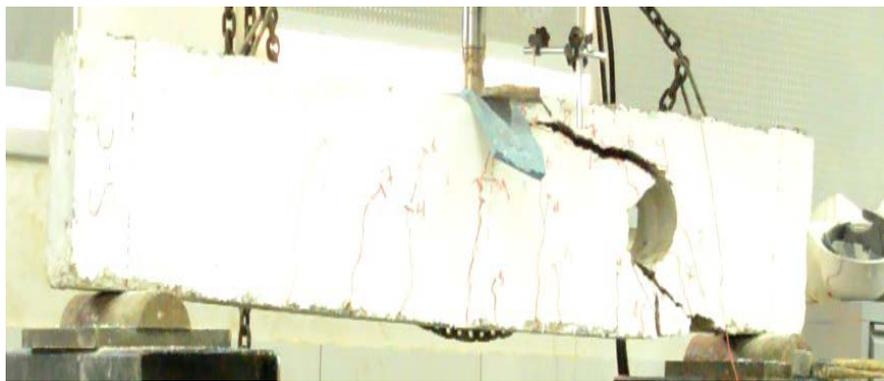
**Figure 12:** crack pattern for beam S-C
