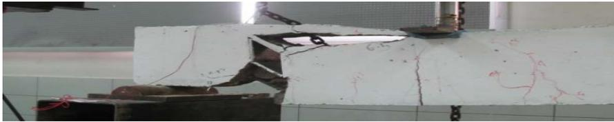
**Figure 15:** crack pattern for beam S-L-Steel
