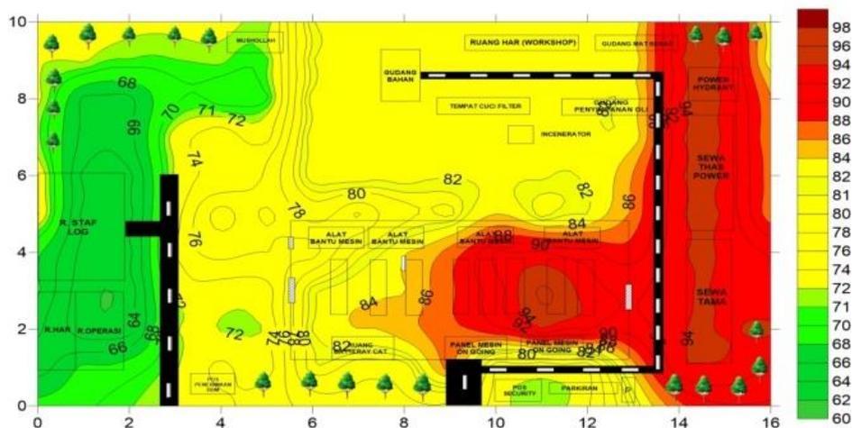
**Figure 1:** Noise Mapping in an Power Plant Company Kendari City in November 2017
