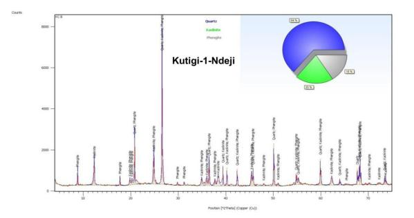
Figure 9: XRD characterization of lower layer of the Kutigi clay showing high quartz and low kaolinitc content
