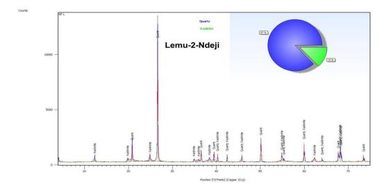
Figure 10: XRD characterization or middle layer of the Lam clay showing very high quanz content
