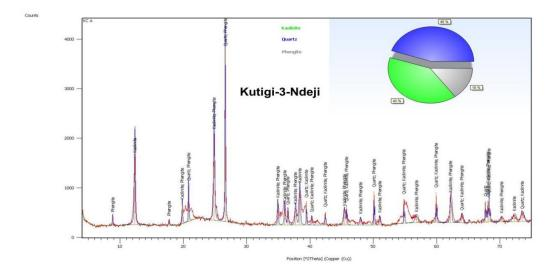
Figure 11: XRD characterization of upper layer of the Kutigi clay showing high kaolinitc content
