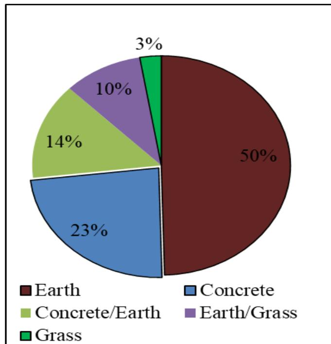
**Figure 5:** Storm water drainage lining
