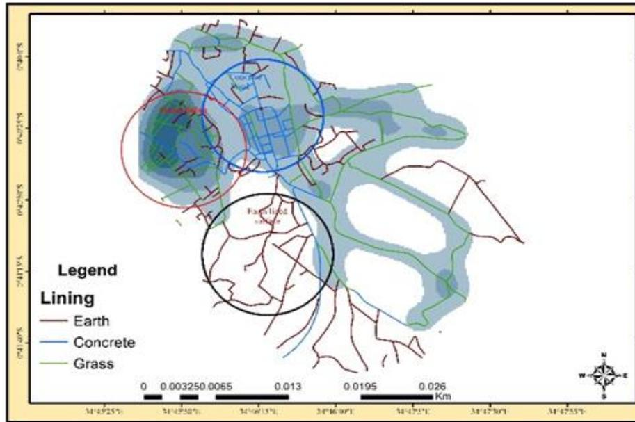
**Figure 3:** Lining material for storm water drainage structure
