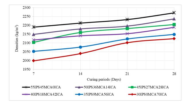
Figure 7: Densities of cured specimens for 450kg/m<sup>3</sup> cement content.
