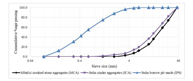
Figure 1: Particle size distribution curves of source aggregates.
