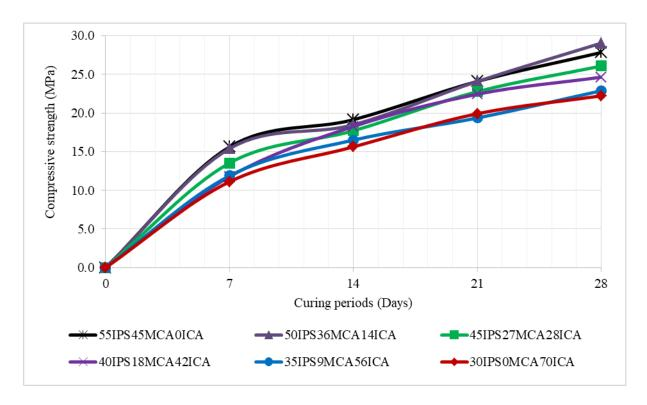
Figure 5: Compressive strength of concrete specimens for 450kg/m<sup>3</sup> cement content.
