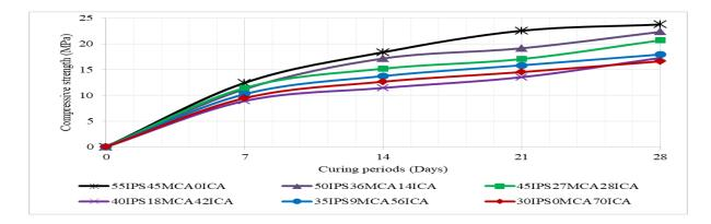
Figure 4: Compressive strength of concrete specimens for 350kg/m<sup>3</sup> cement content.
