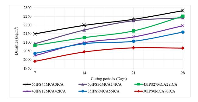
Figure 6: Densities of cured specimens for 350kg/m<sup>3</sup> cement content.
