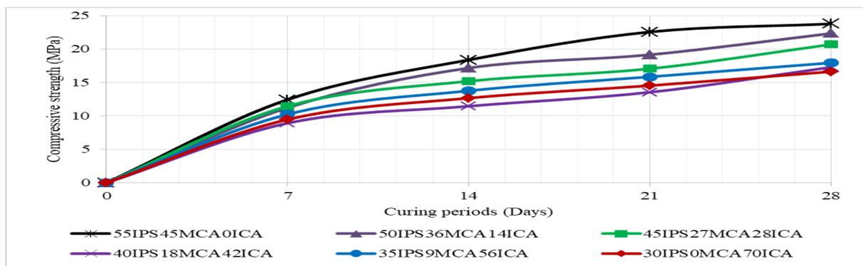
**Figure 4:** Compressive strength of concrete specimens for 350kg/m<sup>3</sup> cement content.
