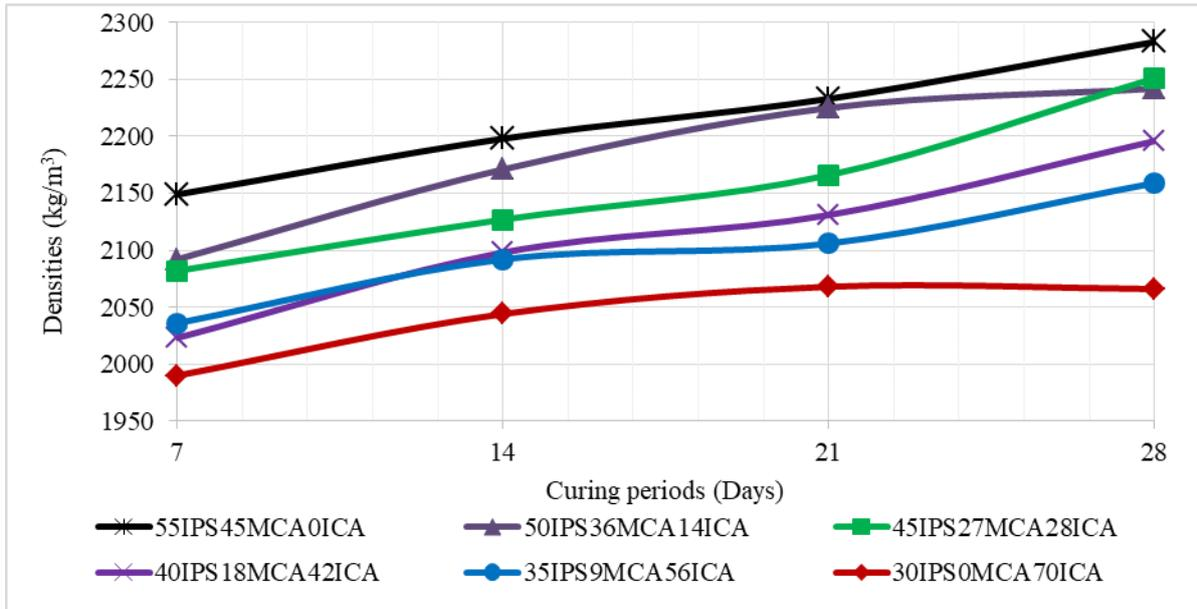
**Figure 6:** Densities of cured specimens for 350kg/m<sup>3</sup> cement content.
