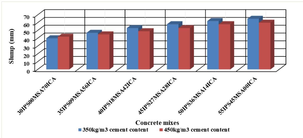
Figure 3: Slump values for fresh concrete mixes.
