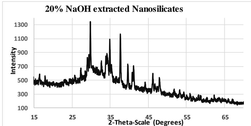
**Figure 6:** XRD pattern of synthesized silicate nanoparticles using 20% NaOH.
