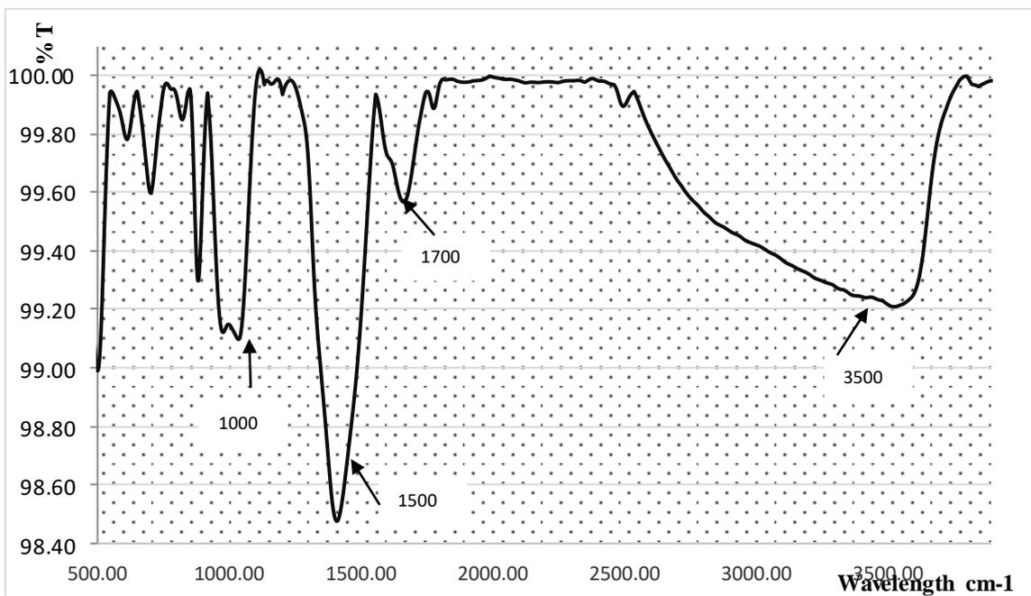
Figure 3: FTIR spectra of synthesized silicate nanoparticles.
