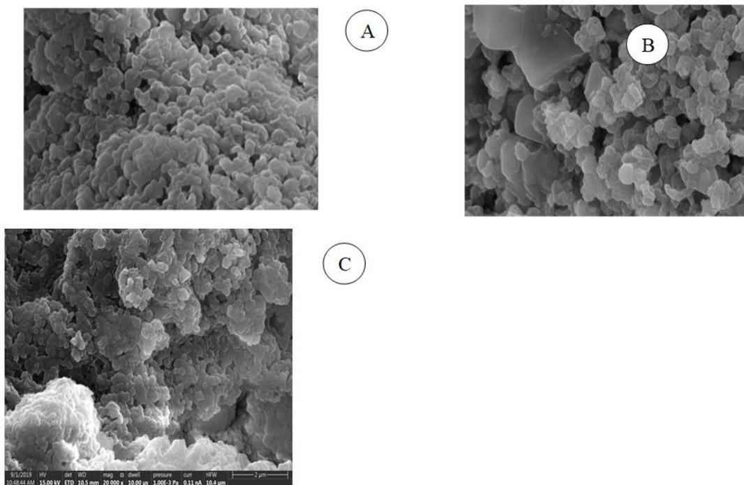
**Figure 4:** FESEM images of synthesized silicate nanoparticles using 20% NaOH (w/v%) (A) 2  $\mu\text{m}$ , (B) 5  $\mu\text{m}$ , and 40% NaOH (w/v%) (C) at 2  $\mu\text{m}$ .
