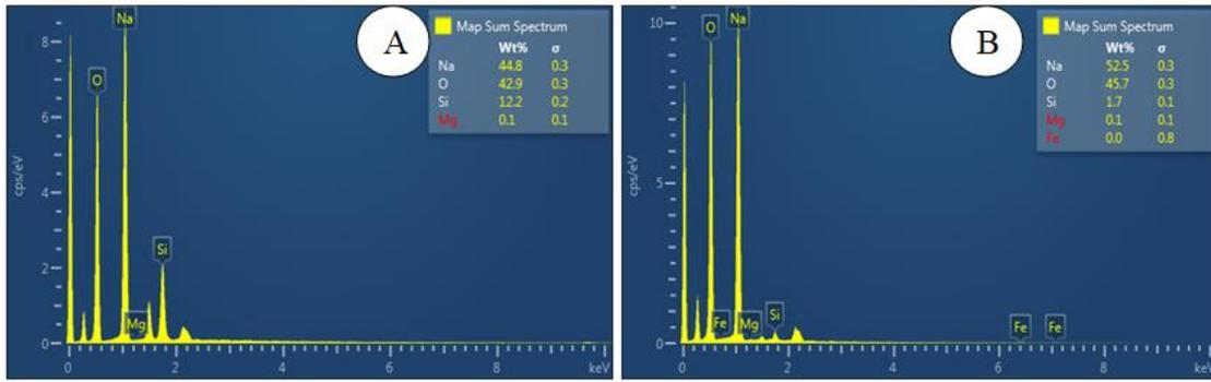
Figure 2: EDX patterns of nanosilicates extract with (a) 20% NaOH and (b) 40% NaOH.
