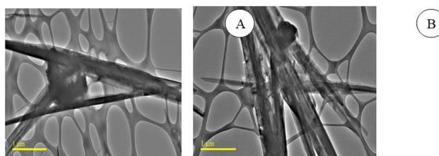
**Figure 5:** FETEM images of synthesized silicate nanoparticles using (A): 20% NaOH (w/v%) and (B): 40% NaOH (w/v %).
