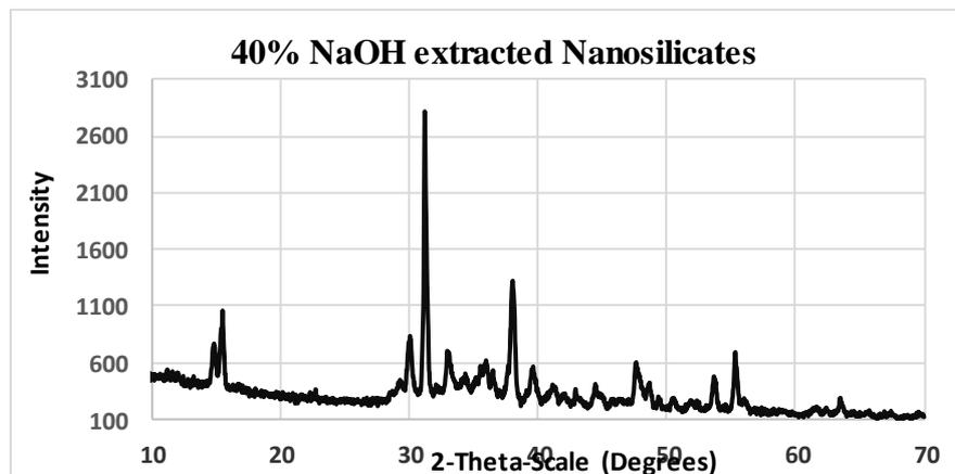
**Figure 7:** XRD pattern of synthesized silicate nanoparticles using 40% NaOH.
