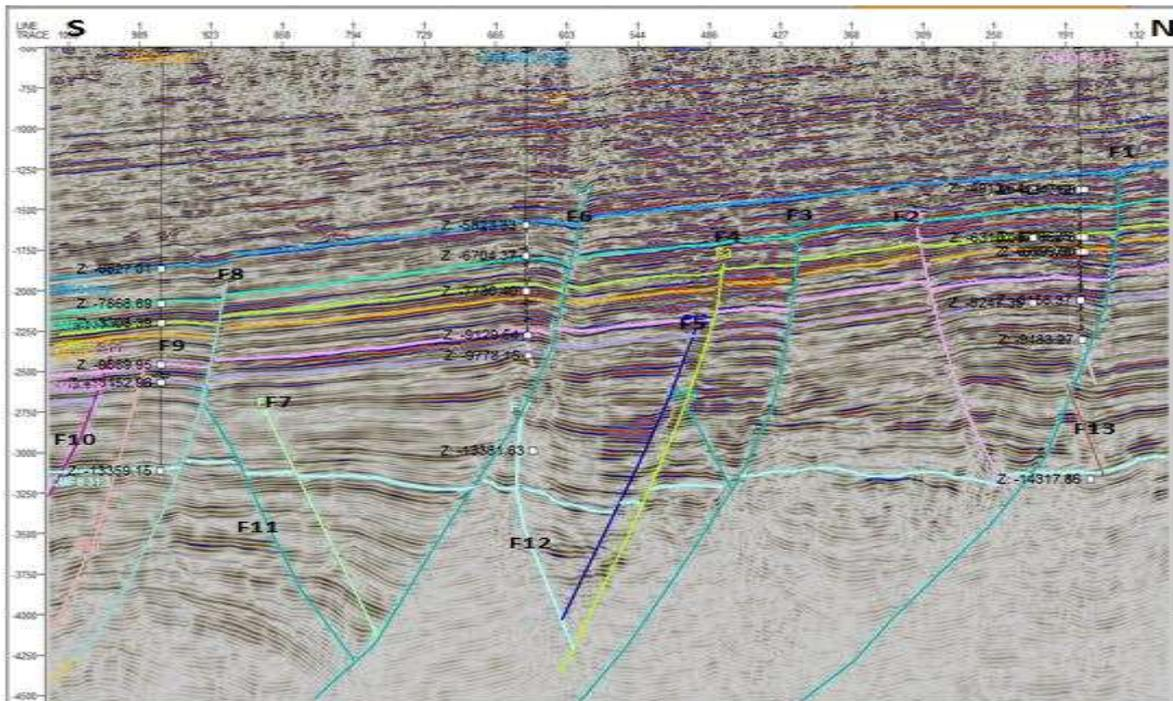
using the identified constrained chronostratigraphic surfaces, in the dip direction. Evidence of faulting was noticed, as the surfaces occurred at varying depth down dip across the wells. Three depositional sequences were identified. Each depositional sequence is bounded above and below by a maximum flooding surface. The details is as summarized in Table 1 and 2.
