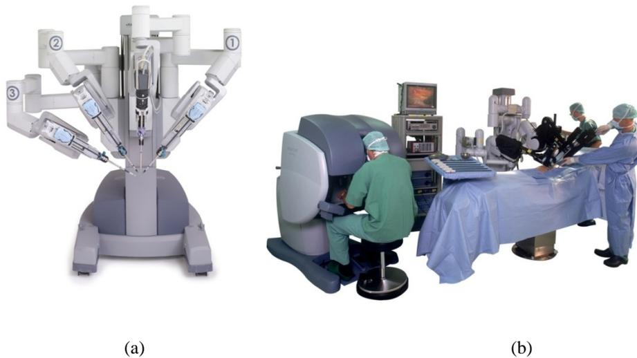
**Figure 2:** (a) Da Vinci surgical system (Courtesy of Intuitive Surgical, Inc.). From left to right: surgeon console, vision system, and patient-side cart; (b) detail of the patient car [2].
