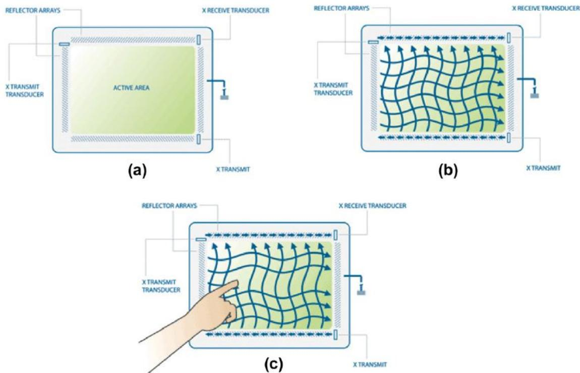
**Figure 1:** Surface acoustic wave touch screen (a). Constitution (b). Non-disturbed acoustic waves pattern, (c) Acoustic wave pattern when touched [2].
