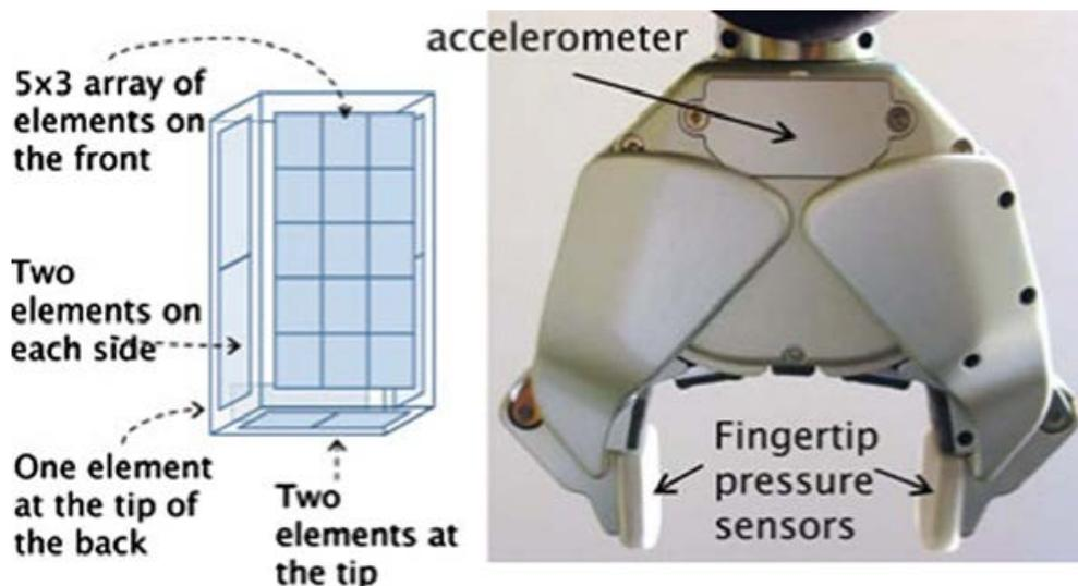
Figure 4: the PR2 robot gripper. The pressure sensors are attached to the robot's fingertips under the silicone rubber coating [2].
