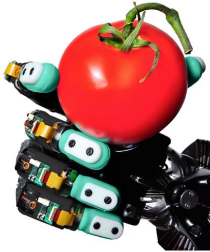
**Figure 5:** SynTouch BioTac tactile sensor [2].
