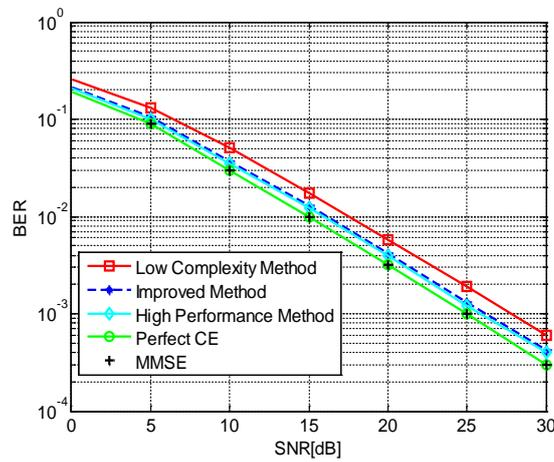
**Figure 7:** BER vs. SNR for the proposed high performance method and other methods under TU-6 Channel
