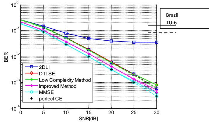
**Figure 6:** BER vs. SNR for the proposed low complexity, improved methods and other methods under 300-Hz Brazil-D and 50-Hz TU-6 channel.
