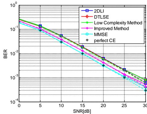
**Figure 5:** BER vs. SNR for the proposed low complexity, improved methods and other methods under 50-Hz Brazil-D and 50-Hz TU-6 channel.
