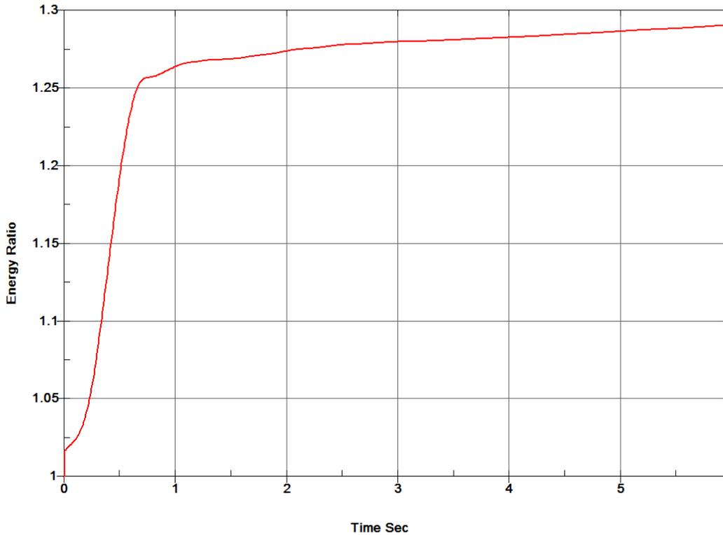
**Figure 18:** Energy ratio for the floating box
