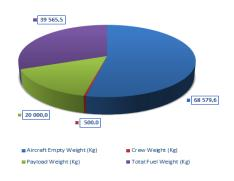
Figure 23: Obtained Weight Allotment – Turboprop Airlifter
