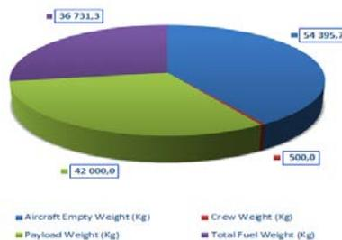
**Figure 16:** Obtained Weight Allotment - Jet Airlifter
