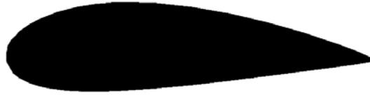
**Figure 25:** Illustration of the NACA 4424
