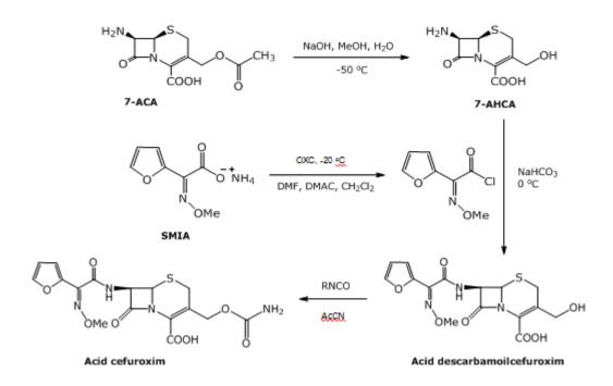
Figure 1: The process for preparation of cefuroxime from 7-ACA and SMIA
