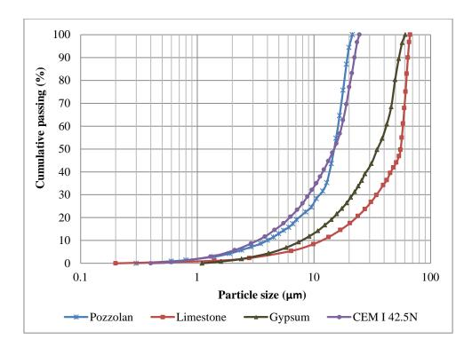
Figure 4: Synthetic particle size distribution of powder materials
