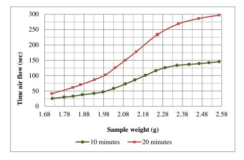
Figure 3: Graphs of time air flows versus weights of pozzolan at different milling duration
