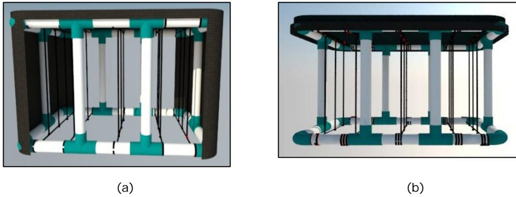
**Figure 3:** Squid attractor; (a) Type 1 (T1) with cover net (Polyethylene 40%) on the upper and both sides and (b) Type 2 (T2) with cover net (Polyethylene 40%) only on the upper side.
