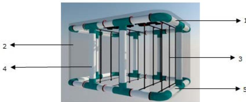
**Figure 2:** Design of squid attractor with PVC pipes material strengthened by cement cast
