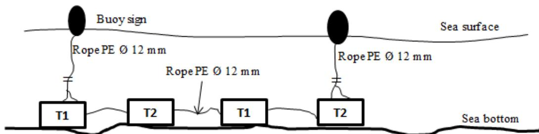
**Figure 4:** Design of 1 series of attractor deployment in the waters
